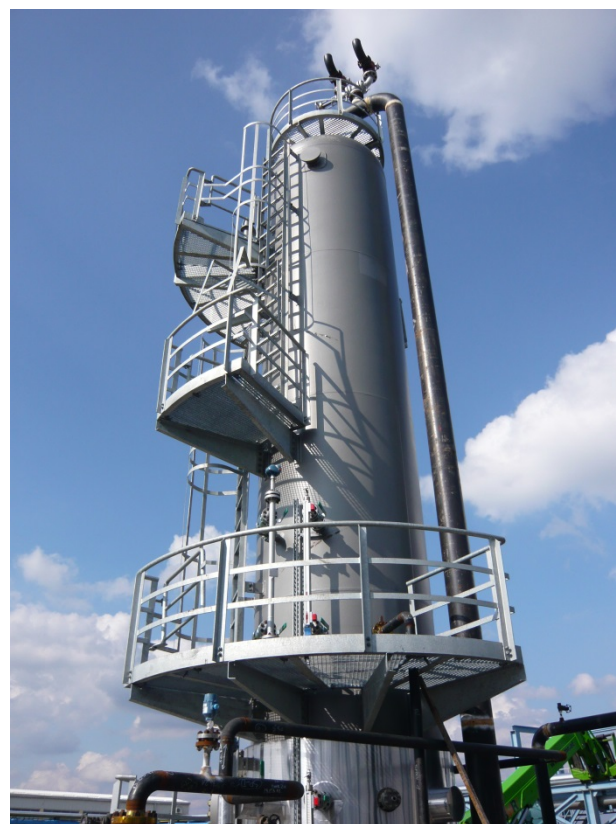
Gas dehydration for 5.000.000 Sm 3 /d and TEG flow of 8.000 kg/h
