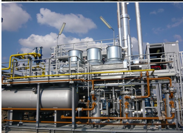
Gas dehydration for 5.000.000 Sm 3 /d and TEG flow of 8.000 kg/h
