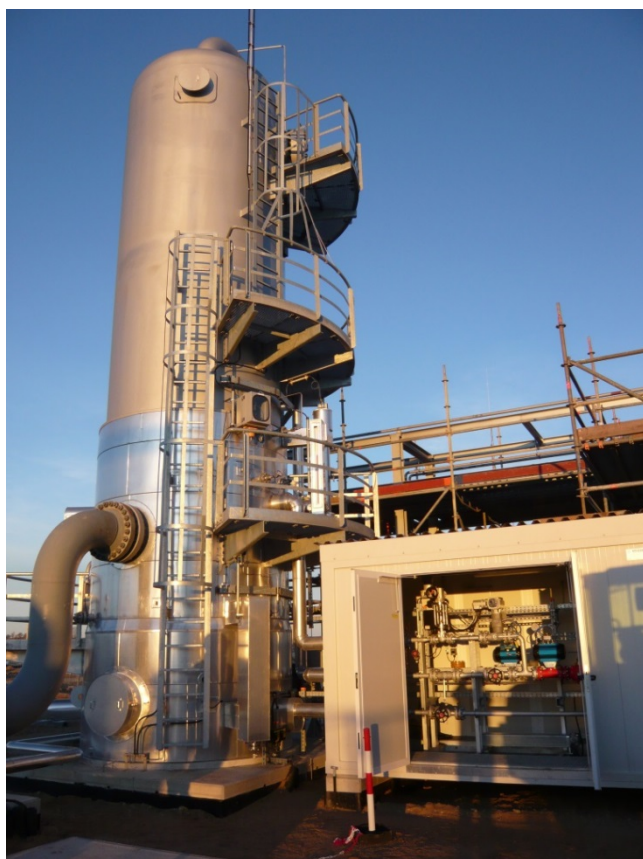
Absorber 400.000 nm 3 /h Vertical incinerator 1000 kW
